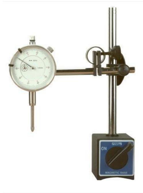
Figure 4.19. Support du comparateur [12]
