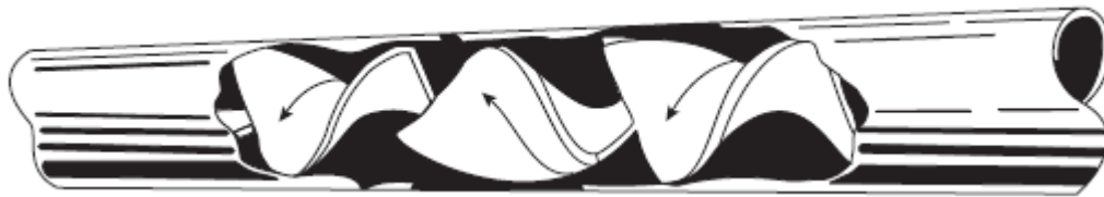
Figure 3.8 Static mixer (Kenics Corporation).
