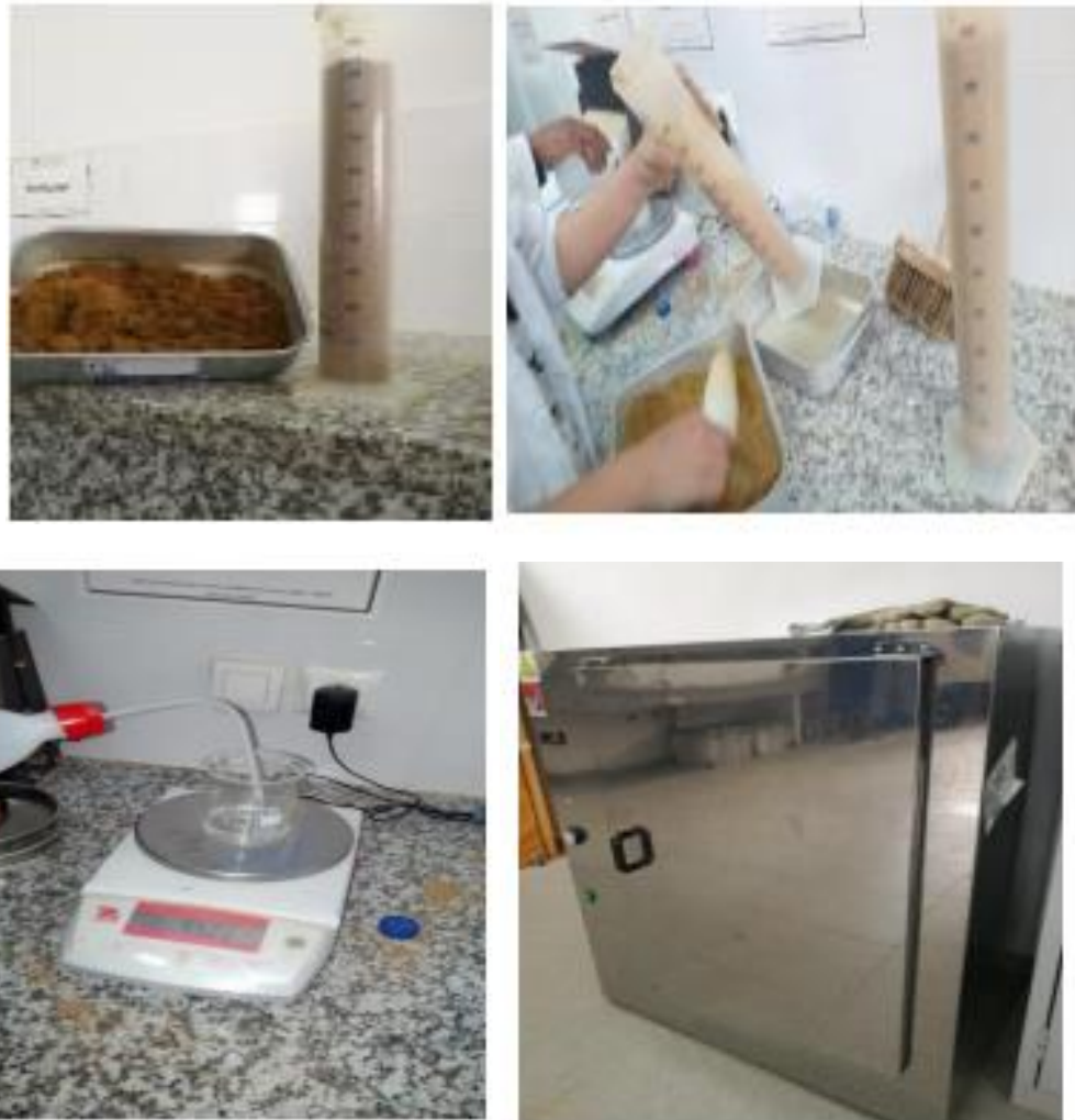
Figure 2.5. Sand bulking test [2]
