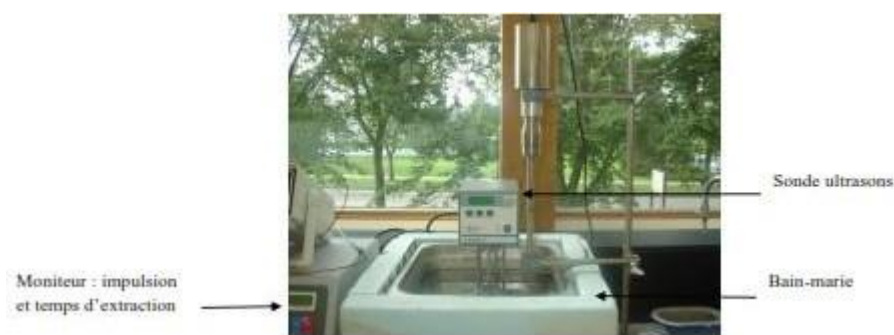
Figure IV.2. Ultrasonic extraction on a laboratory
