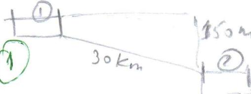
$$\Delta h_{1-2} = \Delta z \Rightarrow \frac{2L}{D} \frac{V^2}{2g} = \Delta z \Rightarrow \frac{8\sqrt{L}}{\pi^2 g D^5} Q^2 = \Delta z.$$
