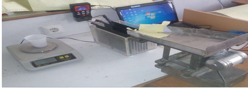
Fig 1: the separation control prototype plus a vibro-transporter, digital scale and LC meter
